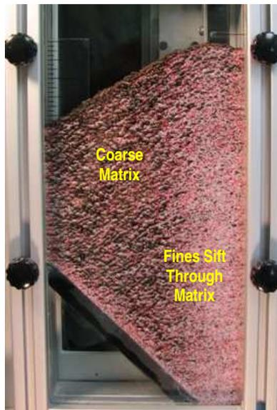
Figure 1. Three-colored sugars in a pile - example of sifting segregation
