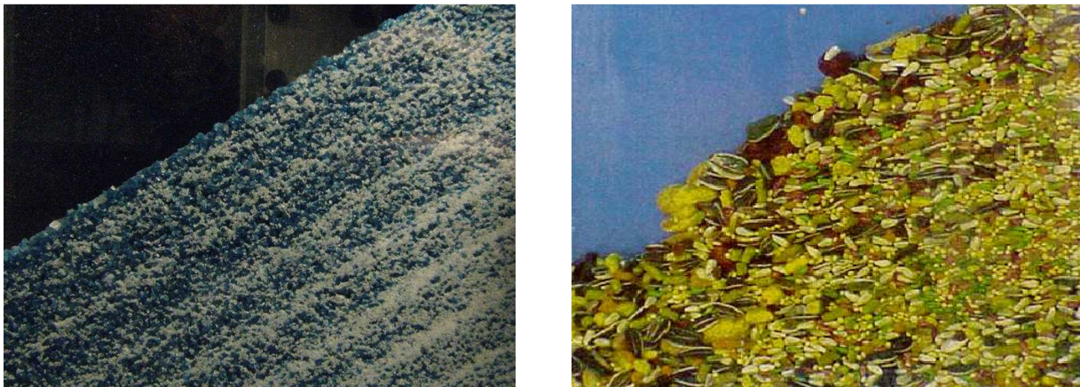
Figure 3. Segregation patterns formed during pile formation in a process
