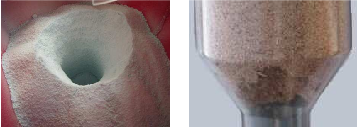
Figure 2. Material hang-up (rathole and arching) of material in a system causes process down-time
