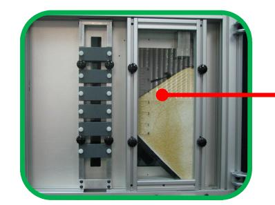
SPECTester front doors reveal the drop chute, testing area, and component trays.
