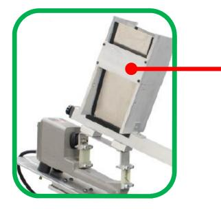
Before filling the SPECTester with the material mixture, samples of the mixture's individual components are placed in the component trays (behind the left door) so that their specific spectral reflectance light-print can be acquired. The adjustable feeder arm can be raised or lowered to simulate actual process drop-height. This makes the test results scalable to the actual production parameters.
